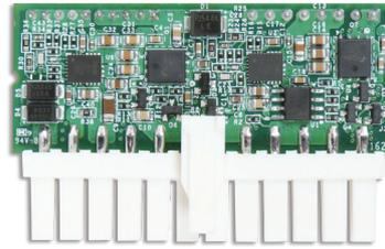
GADIWA-M1120 is a DC-DC converter for socket type. It normally support 96Watts and maximum can reach to 120Watts. GADIWA-M1120 socket type design can save more space and cost, it's not only capability for fan-less system but also suitability for different application. Besides, the converter is made and tested by automatic production line; therefore, it can provide high quality and performance.
