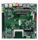
Mini-ITX Form Factor Evaluation Carrier Board for both Type VI Module
