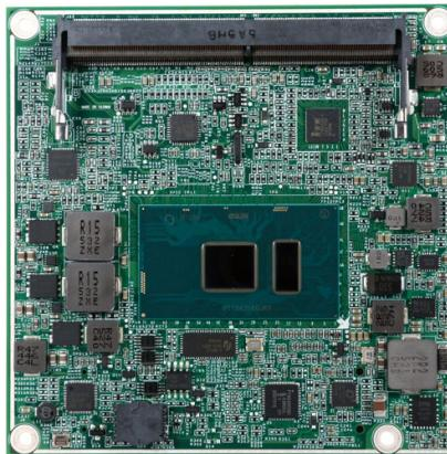
PCOM-B638VG brings three important factors, DDR4 memory support, Gen3 PCIe support, and 30% faster graphic performance. The Gen3 PCIe support provides faster PCIe speed so that the performance of PCIe expansion card will be better. It is crucial for Networking and Medical related applications. The enhanced graphic performance brings 4K support. The OTG support gives customer more flexibilities on developing new applications in different usages.
