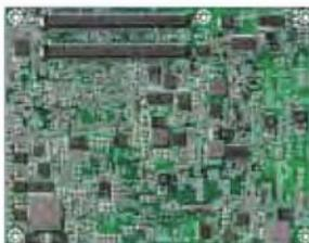
Intel® Sandy Bridge Mobile based Type VI COM Express® with DDR3 SDRAM, VGA, LVDS, Gigabit Ethernet, 6Gbps SATA and USB
