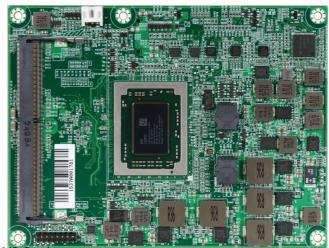
Portwell MEDM-B601 is designed with AMD Quad Core R-Series SoC solution called APU which offers higher computing power and advanced graphic processing ability at lower TDP by introducing AMD 2nd generation heterogeneous system architecture(HSA) for the medical healthcare systems.
