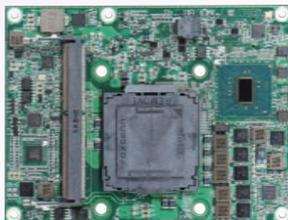
Intel Skylake/Kabylake-S Core i3/ i5/ i7 processor based on Type VI COM ExpressR module with DDR4 SDRAM, VGA, eDP, Gigabit Ethernet, SATA 3.0 and USB
