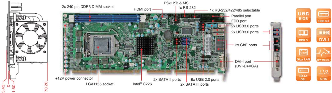
ROBO-8111VG2AR is based on the Intel® C216 chipset and workstation processor sku. Built with flexible PCI express expansion, it's suitable for medical, Factory Automation, and Digital Signage applications.
