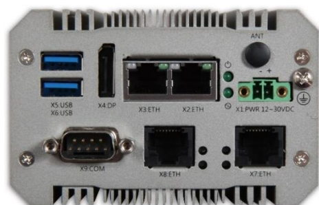
Expanded interface with 2x isolated LAN 1 x RS-232/422/485 (BIOS configurable, 5V & 12V selectable)
