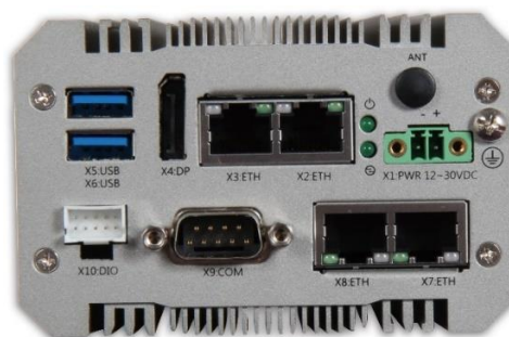
Expanded interface with 4x GPIO, 1x CANBus, 2x Giga LAN
