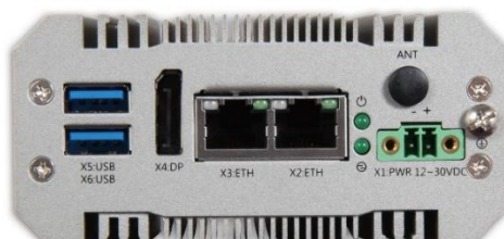
Core interface with 2x USB3.0, 1x DisplayPort, 2xGiga LAN, Power connectors
