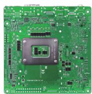
WADE-8213-Q670E is based on Intel® Q670E chipset and 12th/13th Gen Intel® Core™ i9/i7/i5/i3 desktop processors. It supports multiple display outputs, options of legacy features for industrial applications, GPIO ports, dual LAN as well as rich expandability with PCIe Gen5, M.2 M and M.2 E keys. Featuring rich I/O capabilities and advanced connectivity on a smaller and thinner space-saving platform, the Portwell WADE-8213-Q670E is ideal for a wide range of embedded applications.
