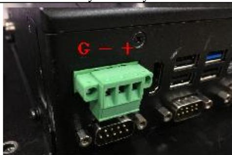
4. Follow pin definition and fix power cable to 3-pin terminal block connector by screw
