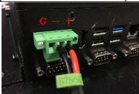
5. Make sure the power supply (12~24V) is connected properly
