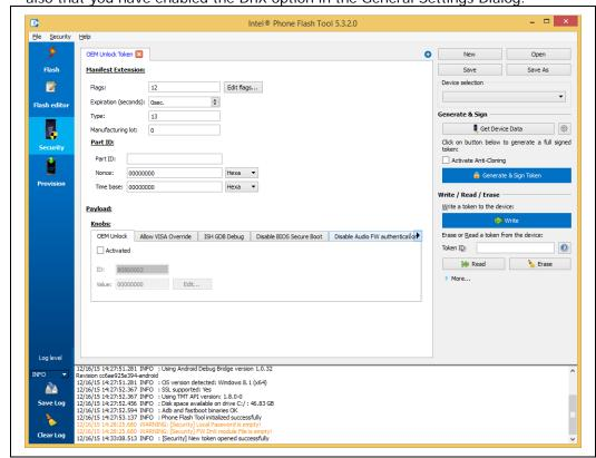
2. In the Payload section, you can set the 'Knobs' for the token. These define what the token allows/disables on the platform. You can check/uncheck the checkbox inside each tab to add the knob to the token, and then edit the value of the token by clicking the Edit button and selecting from the radio buttons inside. Do not attempt to change the value manually. The knobs available vary depending on the token being created. Here is an explanation of the various knobs:
