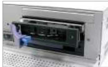
Two Swappable SATA HDD Drives Easy to access HDD drives
