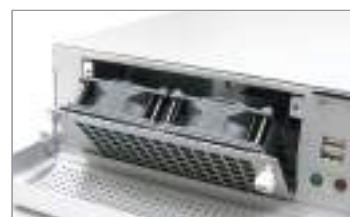
Front Replaceable Air Filters/Fans
