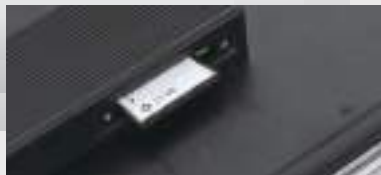
Removable HDD tray and CF cover for easy installation and maintenance.
