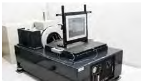
* Compliance with IEC-68 Comply the IEC-68 environmental regulation. The max magnetic force is 1000kgF.
