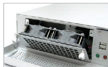
Front Replaceable Air Filters/Fans
