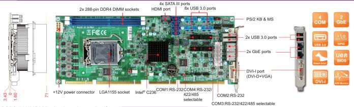
ROBO-8113VG2AR is based on Intel® C236 chipset and workstation processors. Built with flexible PCI express expansions, ROBO-8113VG2AR is suitable for Medical, Industrial automation, and Digital Signage application.
