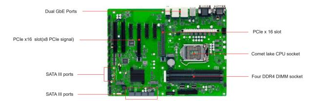
RUBY -D812 is based on Intel® Q470E chipset and Desktop processors including Intel® 10 th Gen Core™ i3/i5/i7 SKU. This board supports DDR4 ,PCIe 4.0, and SATAIII. Those features help you to build high performance and stabile system.
